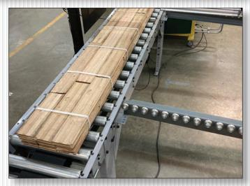
4 Automatic Strapping System The automatic strapping system can be programmed for different strap spacing and different bundle lengths. Strapped bundles are then delivered to the out feed rack for temporary storage.
