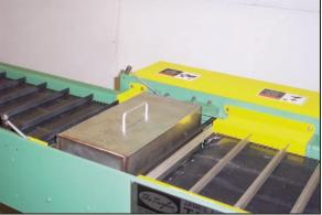
**C) Durability:** The machine is designed with components which stand up to the rigors of a high production gluing operation. In addition, an adjustable safety clutch protects the conveyor chain against damage when careless operation
