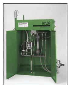
Accurate, Consistent, Adjustable Metering of Components - The Taylor air-actuated, self-priming, positive-displacement piston pumps ensure accurate and consistent metering of components. By adjusting the strokes of the catalyst and waste water pumps, catalyst and waste water-to-resin ratios can be adjusted from 0% to 10%. A fluid flow control valve/pressure gauge system is incorporated to provide for very precise calibration of the Mixer.
