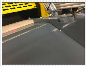
Board Width Sensor reading board
