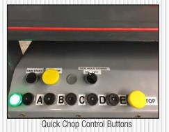
Quick Chop allows the operator to stand at one position and mark defects with a fluorescent crayon. The Quick Chop determines the cut solution based on the defect crayon marks and the Cut Bill. Special marks can even be used for grading purposes. This allows multiple Cut Bills to be used on the same board.
