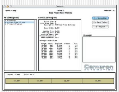
Main screen of Quick Chop Software showing current cut bill and current board being chopped.
