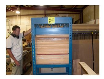
**#78H-12-42-40 Vertical Press** 12" Wide x 42" Long x 40" Opening 10 ton Capacity Press Modular Design Allows Expansion For Longer Parts
