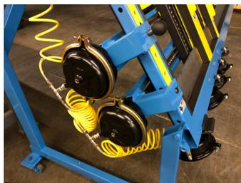
Includes (4) vertical and (2) horizontal clamps. Also includes center vertical rail for multiple cabinet door squaring.
