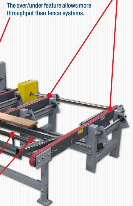
The Quick Rip is fenceless. Boards are skewed (if necessary) for the operator to see under the laser lights. They are then picked up and fed into the saw.
