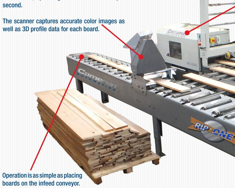
Compact design allows one operator to feed and tail the system, reducing labor or easily integrate with automated material handling system.
