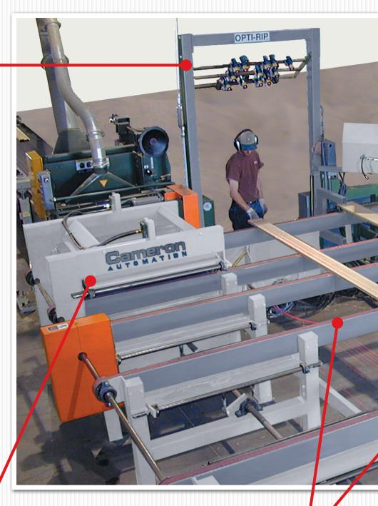
Pinch Roll Assembly is used to lift boards from the belts and deliver to the saw without changing the rip solution.
