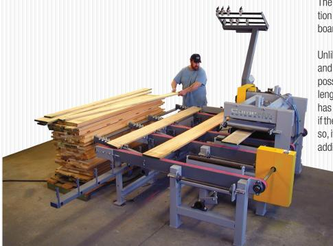
The Quick Rip System is a mid-range Optimization System for shops ripping 6,000 - 18,000 board feet per shift.
