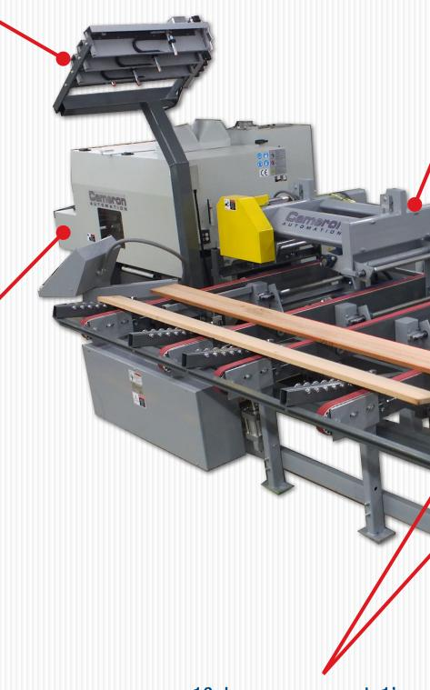
16 laser sensors at 1' increments measure the length, width and shape of every board.
