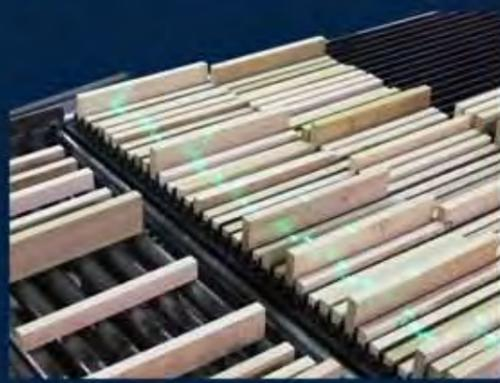
Scanning is based on line lasers at high angles being read from USB based array cameras. As many as 34 staves are measured at any time for each panel solution. Final solutions within +/- 0.50" up to 40" wide panels. The final stave groups are kept together and fed to a customer supplied glue wheel.
