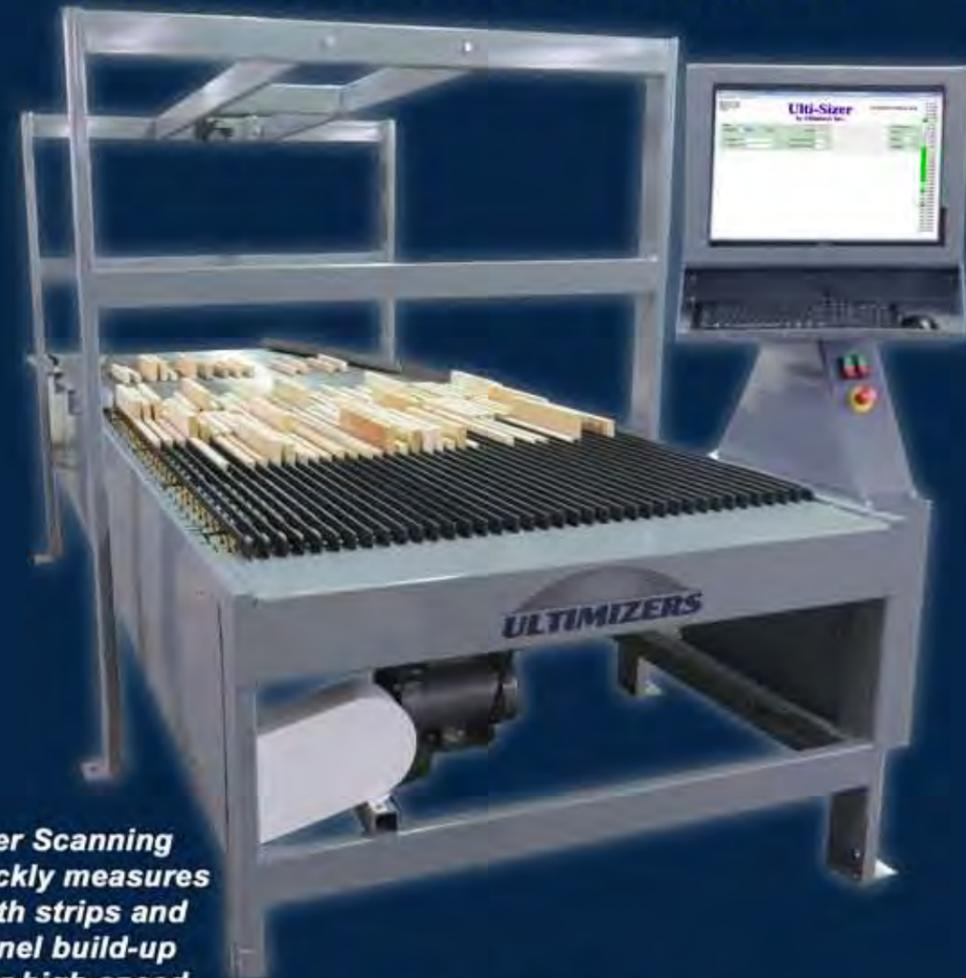
*The Ulti-Sizer Scanning System Quickly measures random width strips and provides panel build-up solutions for high speed panel glue-up operations or for operations needing solutions for wide panels.*
