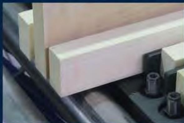
Heavy duty air operated stops resist dust and debris while maintaining quick and consistent operation.
