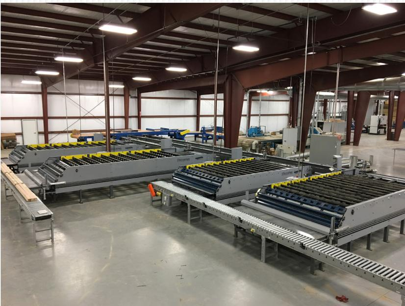
Four Flooring Nesters at a Engineered Flooring Plant in Tennessee.
