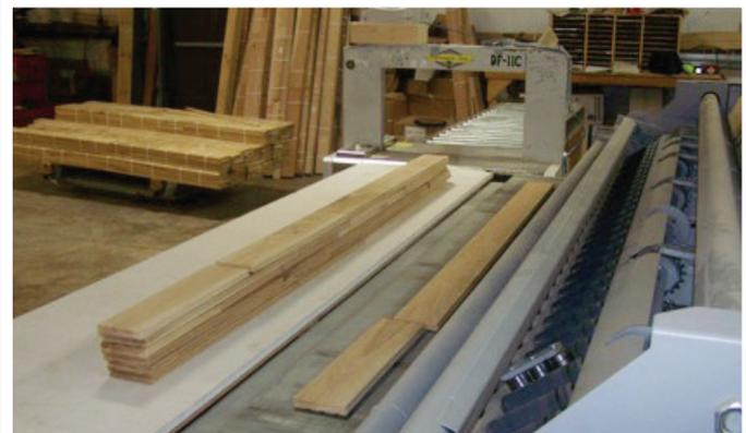
**Strips are accumulated into rows. Rows are accumulated into layers. Layers are accumulated into bundles.**
