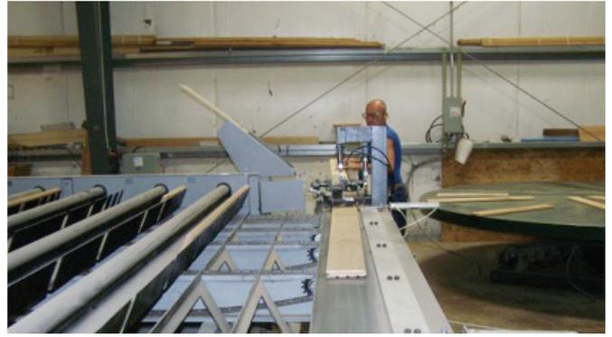
**Strips of flooring are singulated and measured for length before being released into the main machine.**
