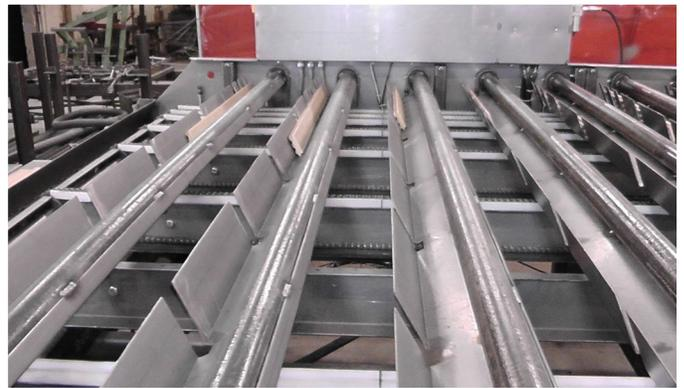
**Strips are scooped off of main conveyor and stored until needed.**
