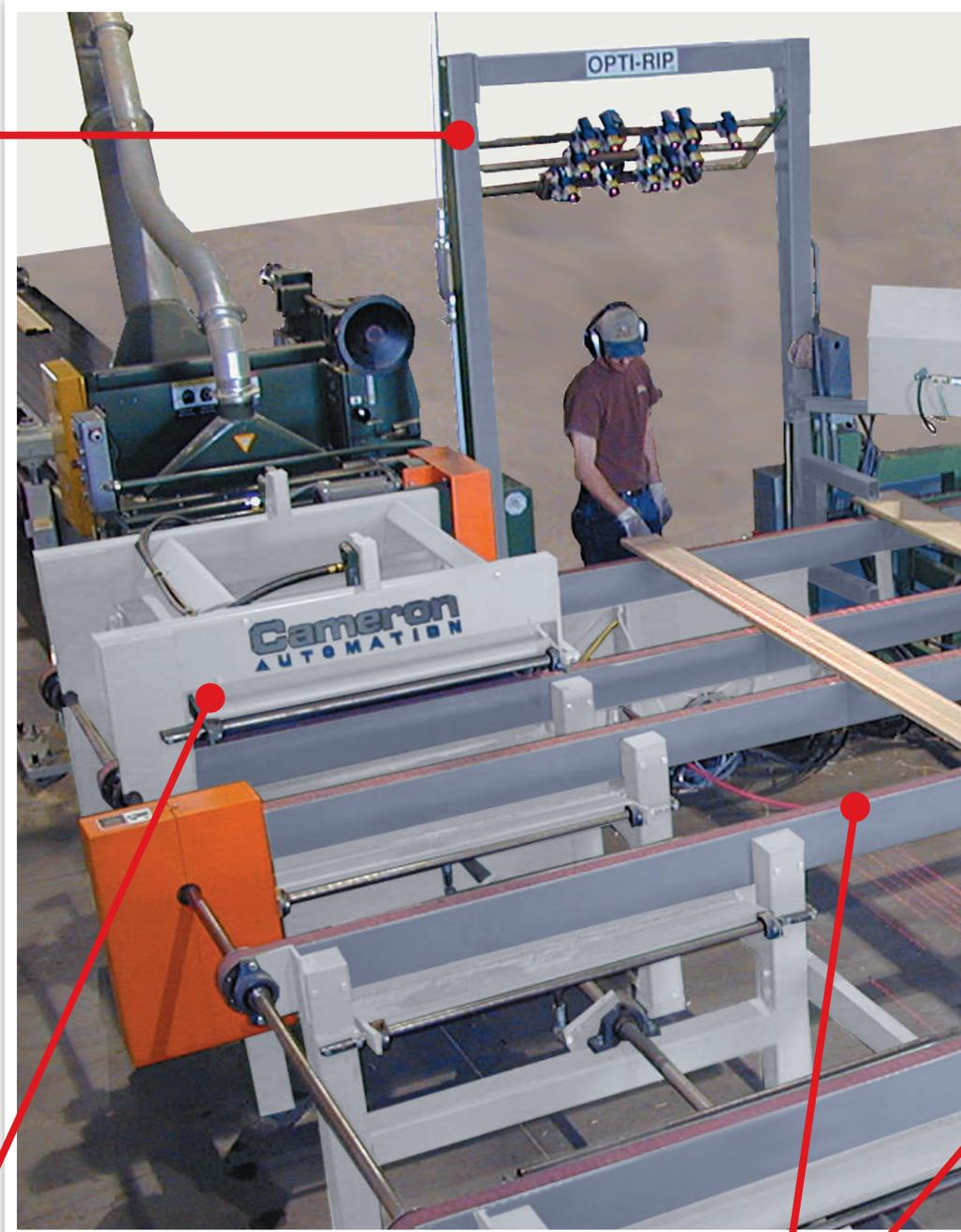
Pinch Roll Assembly is used to lift boards from the belts and deliver to the saw without changing the rip solution.
