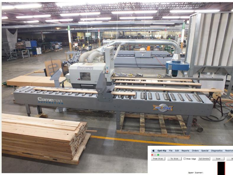
The Rip-One with a 2 Moving Blade Saw
