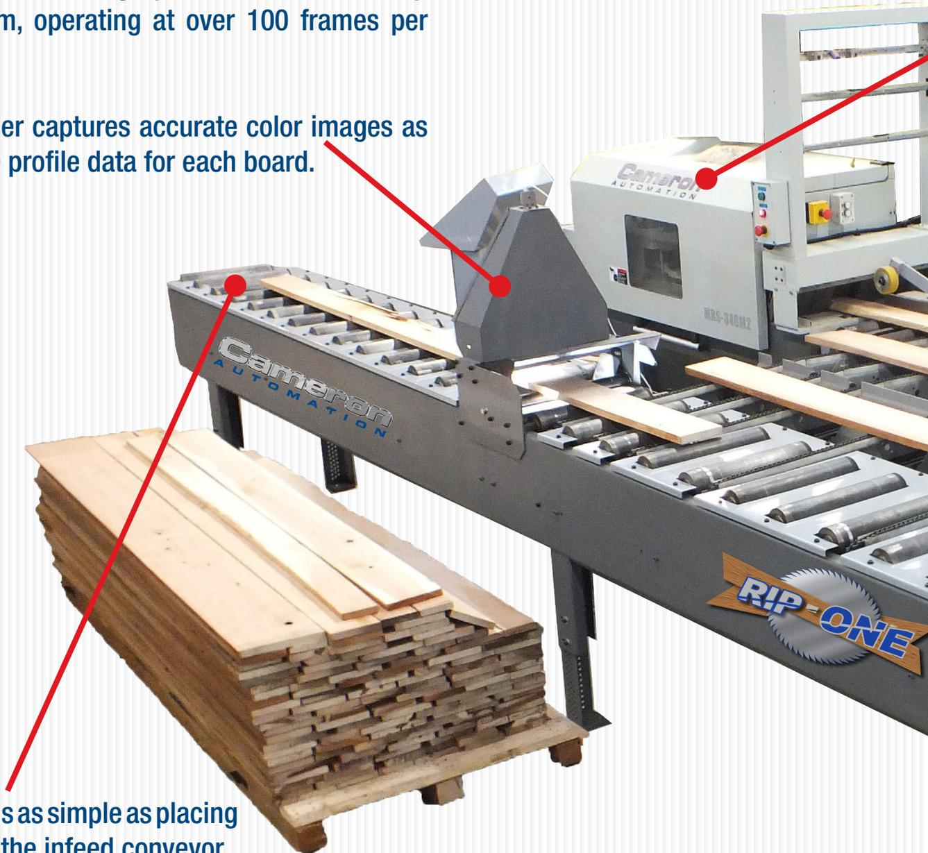
Operation is as simple as placing boards on the infeed conveyor.
