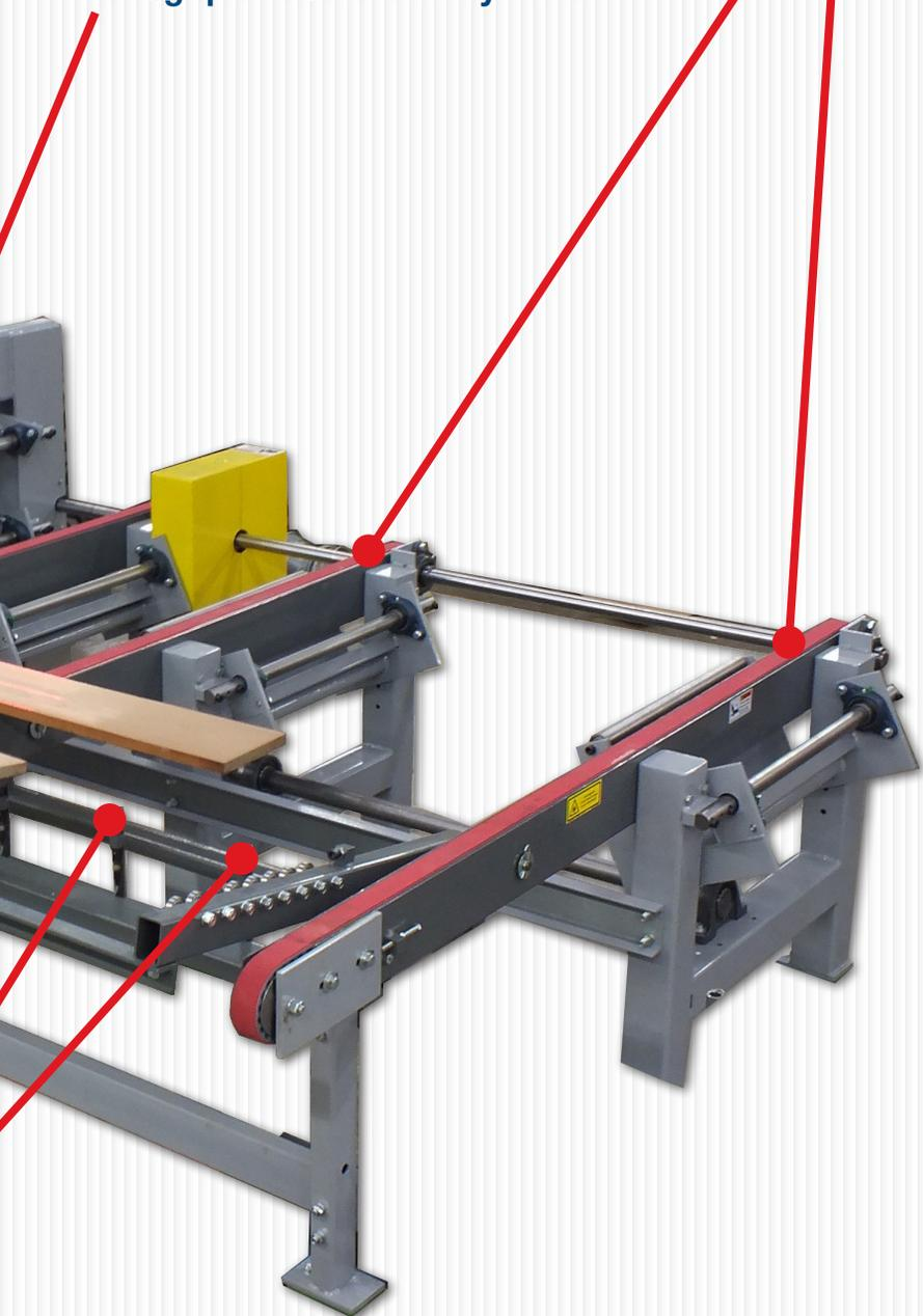
The Quick Rip is fenceless. Boards are skewed (if necessary) for the operator to see under the laser lights. They are then picked up and fed into the saw.
