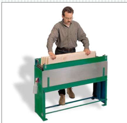
The Plate Spreader provides an accurate and efficient glue spread. It works well with our Clamps to quickly apply glue to multiple boards. A perforated aluminum grid, 8" x 48", rises from the stainless steel glue container by a foot activated pedal to provide the correct amount of adhesive. Boards over 48" can be 'dipped' twice. An aluminum cover for the glue container extends glue use. It is fast, convenient, easy to use and clean.
