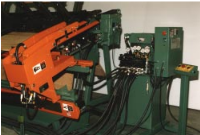
View of the Control Cabinet which houses the "Smart Clamp" controller.
